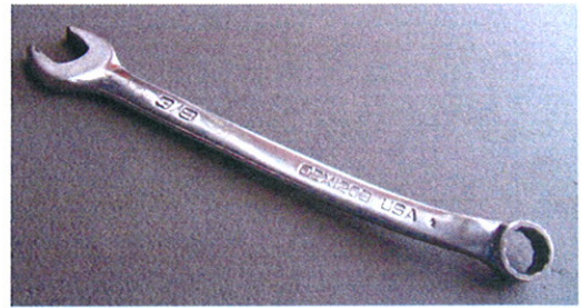
Photo 2: Bent &amp; Twisted Body
