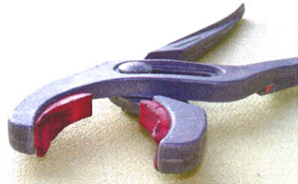
Photo 3: Worn Plastic Jaws Grips
