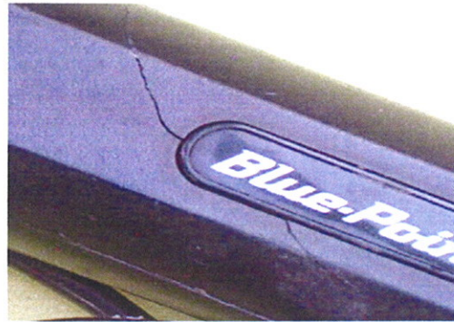
Photo 2: Worn & Cracked casing
