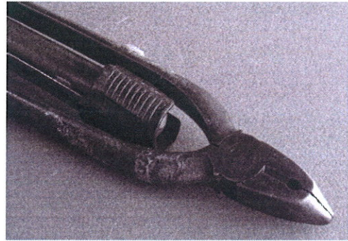
Photo 4: Worn vinyl or rubber casing.
