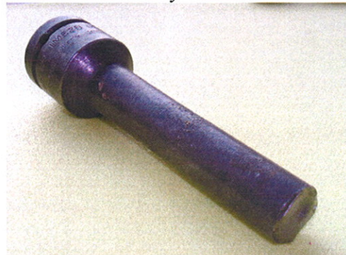
Photo 1: Broken Impact Adaptor.
