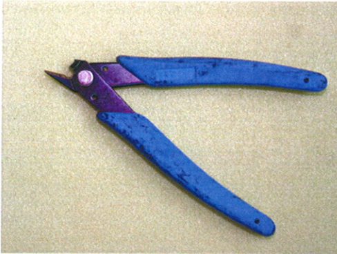
Photo 1: Jaw Broken at Base
