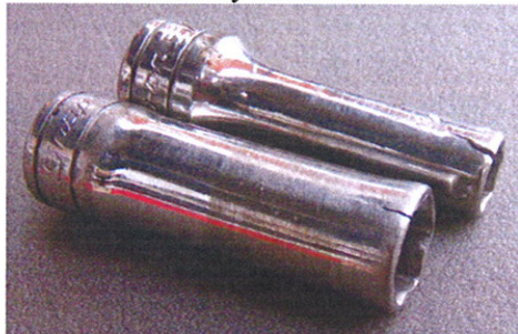
Photo 1: Cracks at Teeth End
