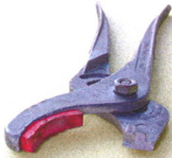
Photo 2: Jaw broke at base.
