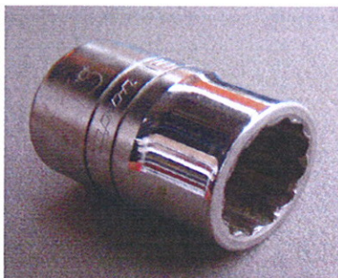
Photo 1: Wear &amp; Tear at Teeth
