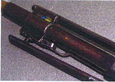
Photo 3: Worn or damaged locking mechanism.
