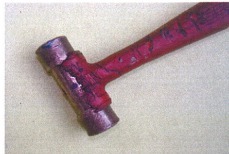
Photo 2: Wear & Tear on Soft Head
