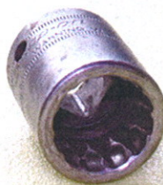
Photo 2: Wear &amp; Tear at Teeth
