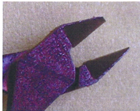
Photo 1: Jaw tip chipped-off.
