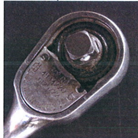
Photo : Cover Plate broken or cracked
