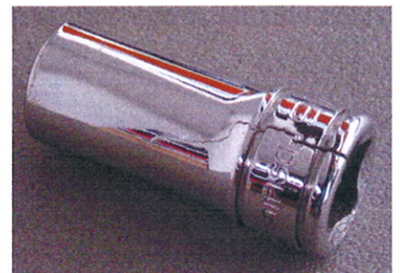
Photo 3: Crack at Drive End
