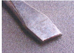
Photo 1: Chipped at Tip.
