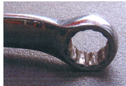
Photo 4: Worn-off Teeth (Wear &amp; Tear)
