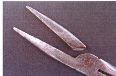
Photo 2: Broken at Jaw Base
