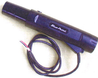
Photo 1: Power cord cut.
